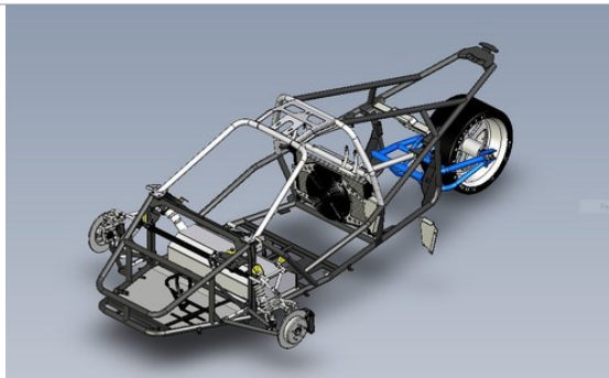
Frame chassis of a SilverLight reverse-trike Source: SilverLight Electric Vehicle Inc.
